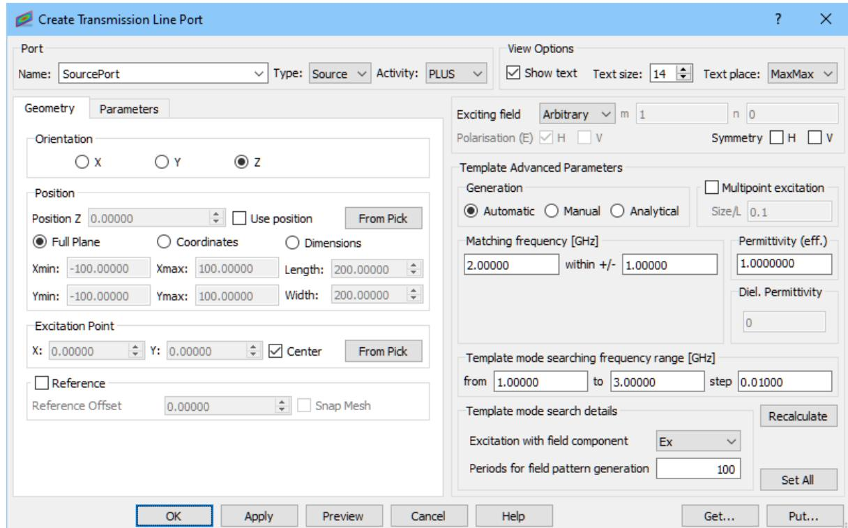
We set the name of the port to *SourcePort*. The default *Type* and *Activity* of the port are properly set for this case. The *Orientation* should be changed to Z. *Full Plane* option sets the port dimensions equal to the bounding dimensions of the entire project in the directions perpendicular to the port orientation what is suitable in this case. We uncheck the *Reference* option – it is not necessary since we do not calculate S-Parameters.
