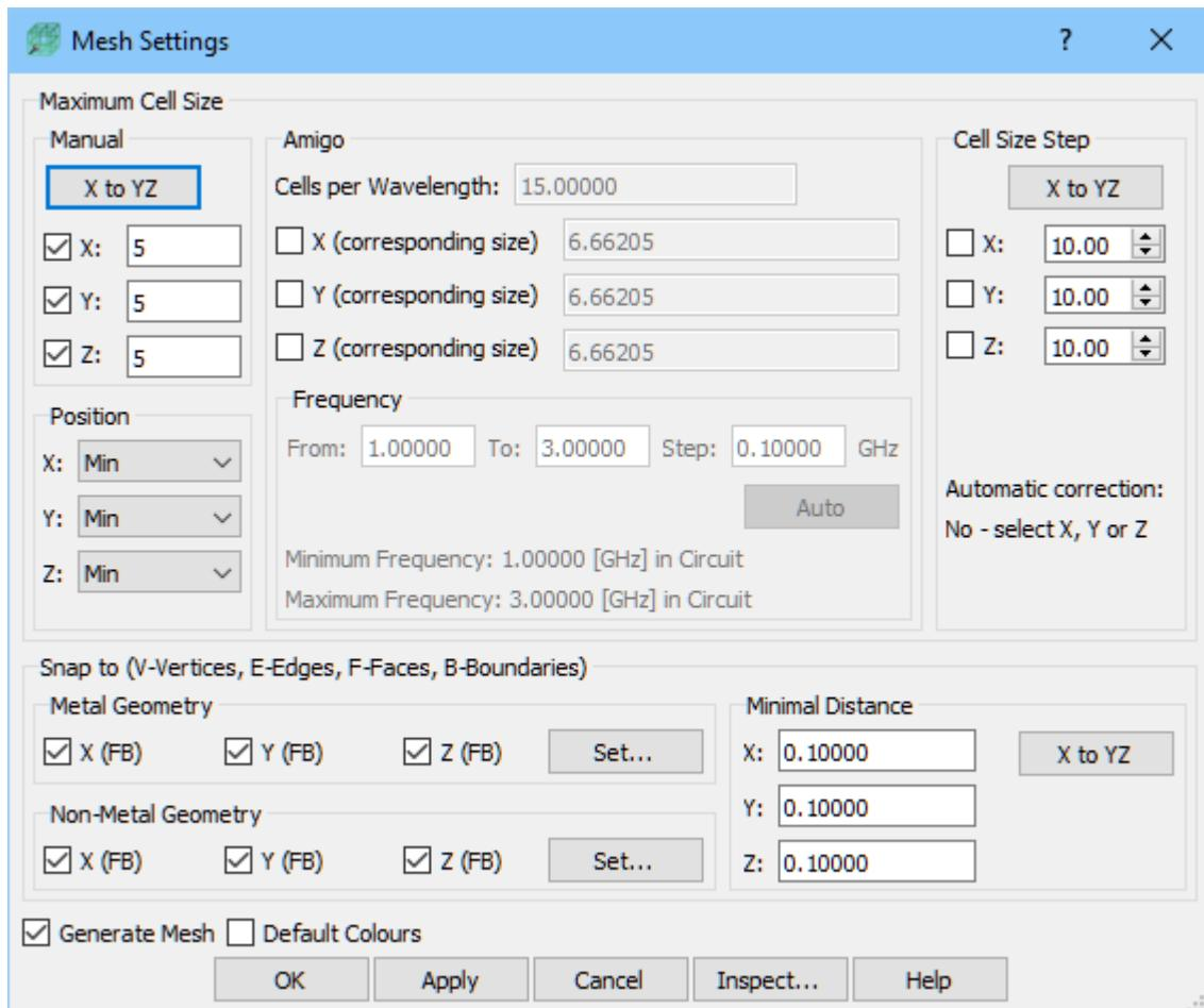
We set 5mm cell sizes in X, Y and Z direction. The meshing will be enforced in the entire project space.
