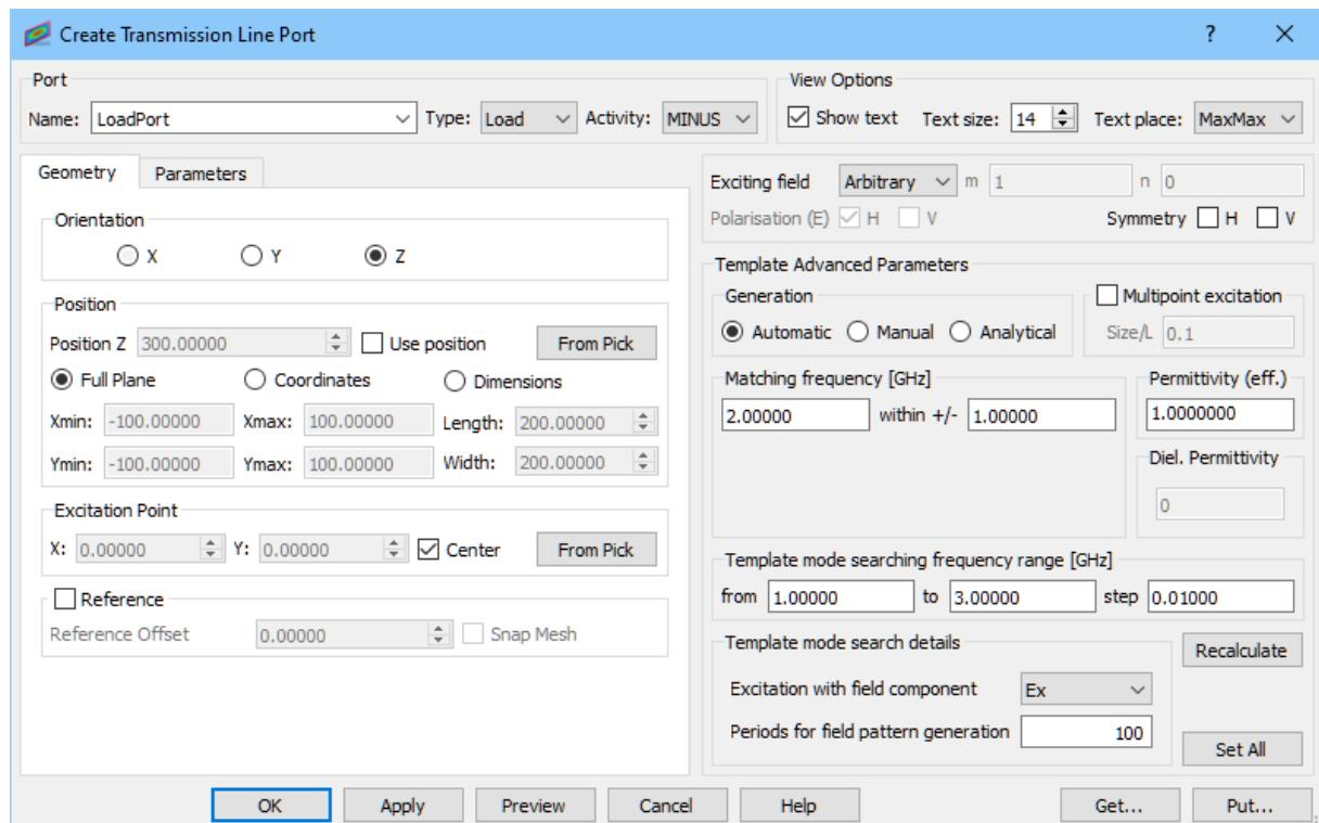
We set the name of the port to *LoadPort*. The default *Type* of the port is properly set for this case. The *Orientation* should be changed to *Z*. We should also change *Activity* to *MINUS* (please note that when *Full Plane* option is checked, port will change its position to the opposite side of the project). We uncheck the *Reference* option – it is not necessary since we do not calculate S-Parameters.
