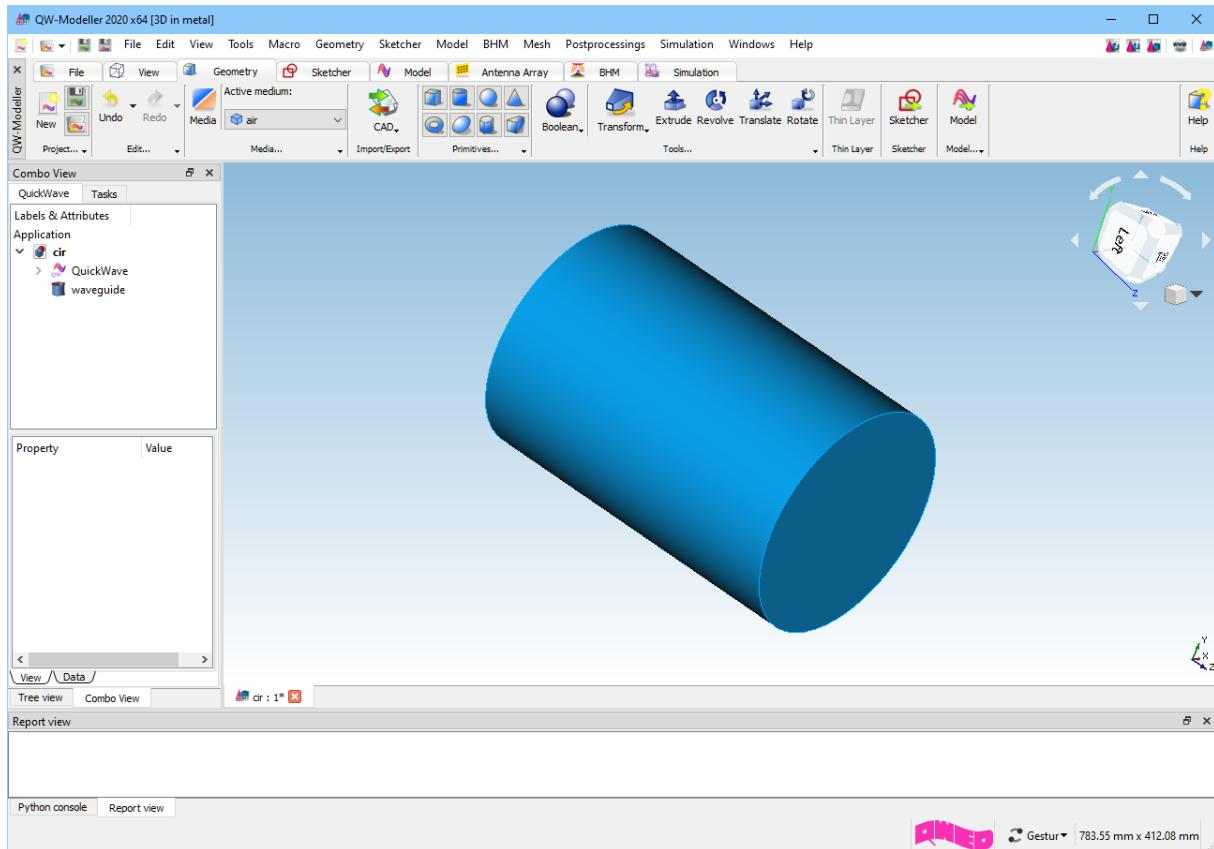
For better visualisation of the inside of the waveguide, we change its transparency by selecting *waveguide* object on the *Tree View*, and changing *Transparency* in the *View tab* in *Property Editor* to 50.
