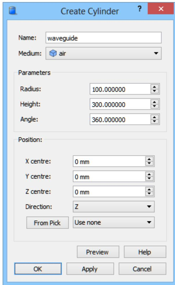
We set the object's name to "waveguide". From the *Medium* combo box we choose air. Now we can proceed to setting the dimensions of the waveguide's inside according to the picture above. With *Position* set to (0,0,0) the waveguide will be drawn so that its centre is placed at these coordinates. After pressing *OK* button the waveguide's inside appears in the project.
