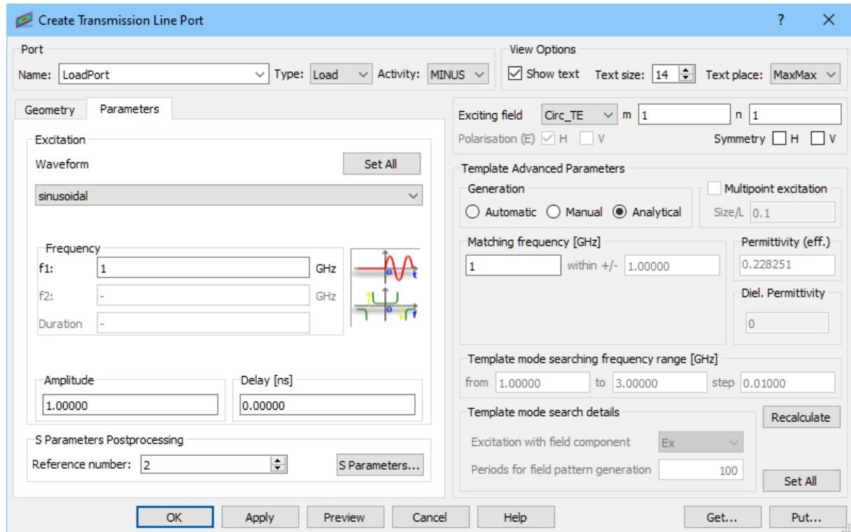
In the *Parameters* tab we set sinusoidal excitation at 1 GHz. We excite the structure with a fundamental TE<sub>11</sub> mode by setting *Analytical* generation, choosing *Circ\_TE* from the *Exciting field* and setting *m* and *n* indexes to 1. Pressing *OK* button accepts the settings.
