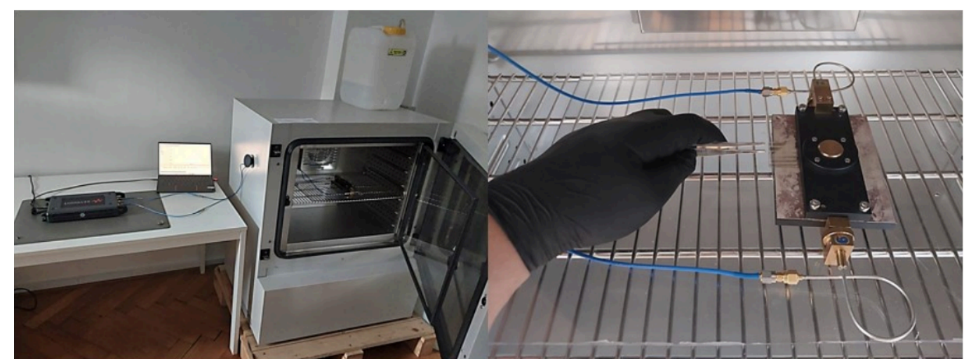
10 GHz Split Post Dielectric Resonator in Climate Chamber with inserted 4H-SiC treated by Ion implantation
