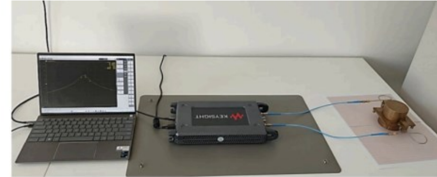
Dual mode RuDR measurement setup which also includes VNA and laptop with dedicated software.
