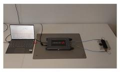
GO and rGO samples under test on 5GHz SiPDR measurement setup which also included a VNA and a laptop with dedicated software.
