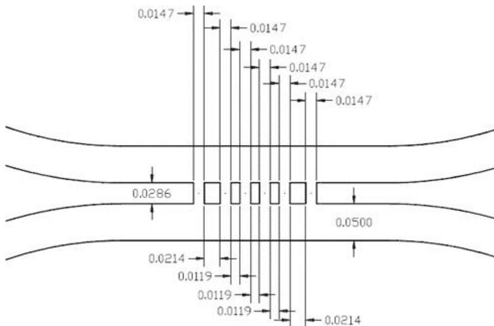
**Fig. 1** Scheme of waveguide quadrature hybrid proposed in [1]. The hybrid is based on WR-10 waveguide and contains six branch lines. All dimensions are given in inches.
