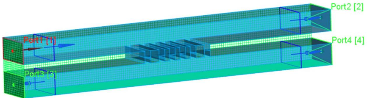
**Fig. 2** Simulation model of WR-10 waveguide quadrature hybrid with six branch lines, prepared in QW-Modeller [3].
