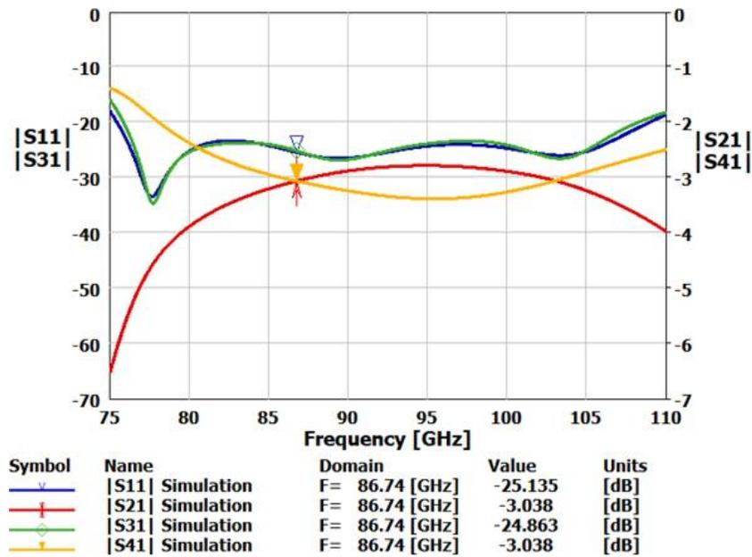
**Fig. 4** Magnitude of reflection ( $|S_{11}|$ ) and transmission ( $|S_{21}|$ ,  $|S_{31}|$ ,  $|S_{41}|$ ) coefficients of WR-10 quadrature hybrid computed with QuickWave 3D.
