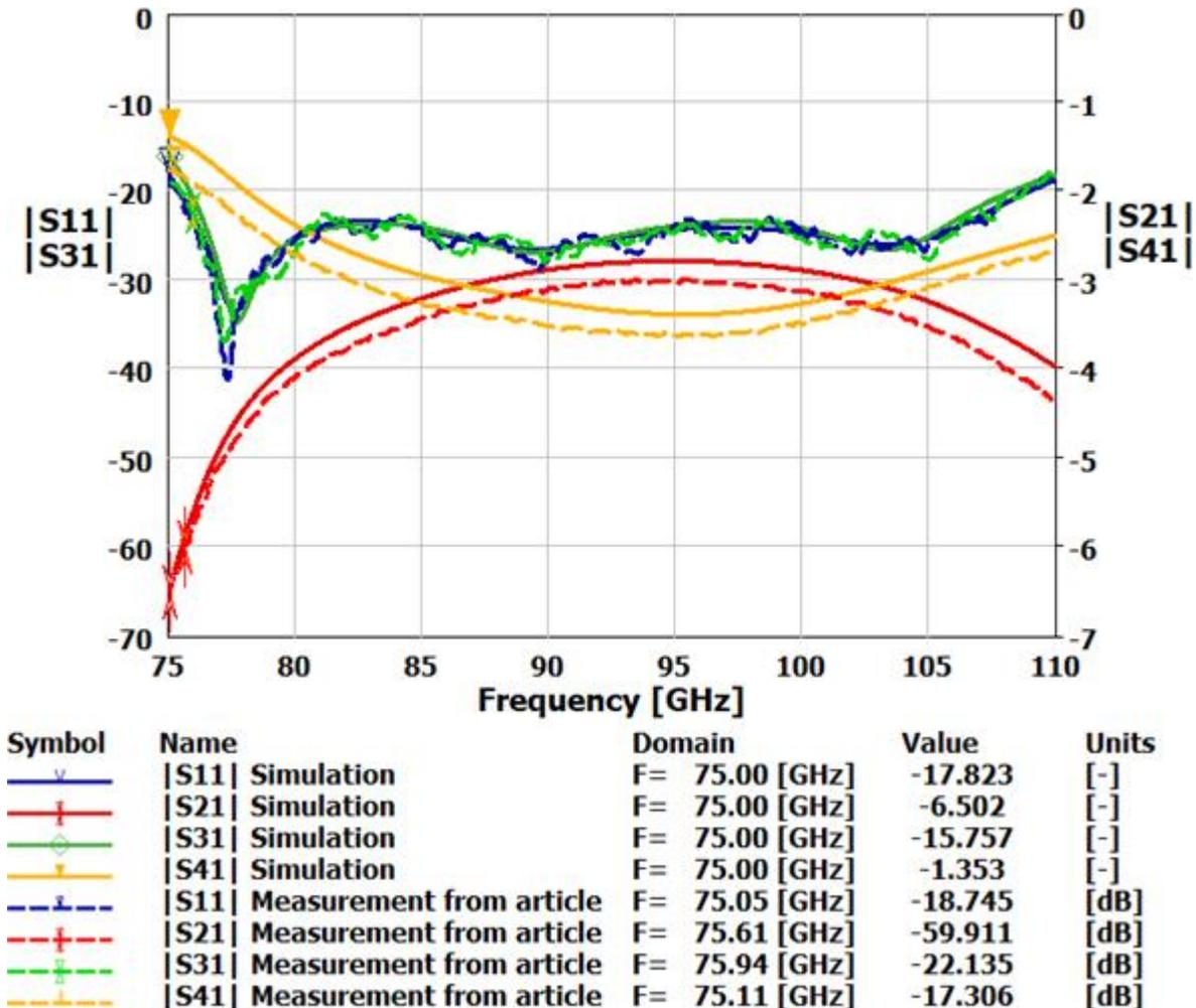
Fig. 9 The magnitude of reflection ( $|S_{11}|$ ) and transmission ( $|S_{21}|$ ,  $|S_{31}|$ ,  $|S_{41}|$ ) coefficients of WR-10 quadrature hybrid – simulated data and measurements from [1].
