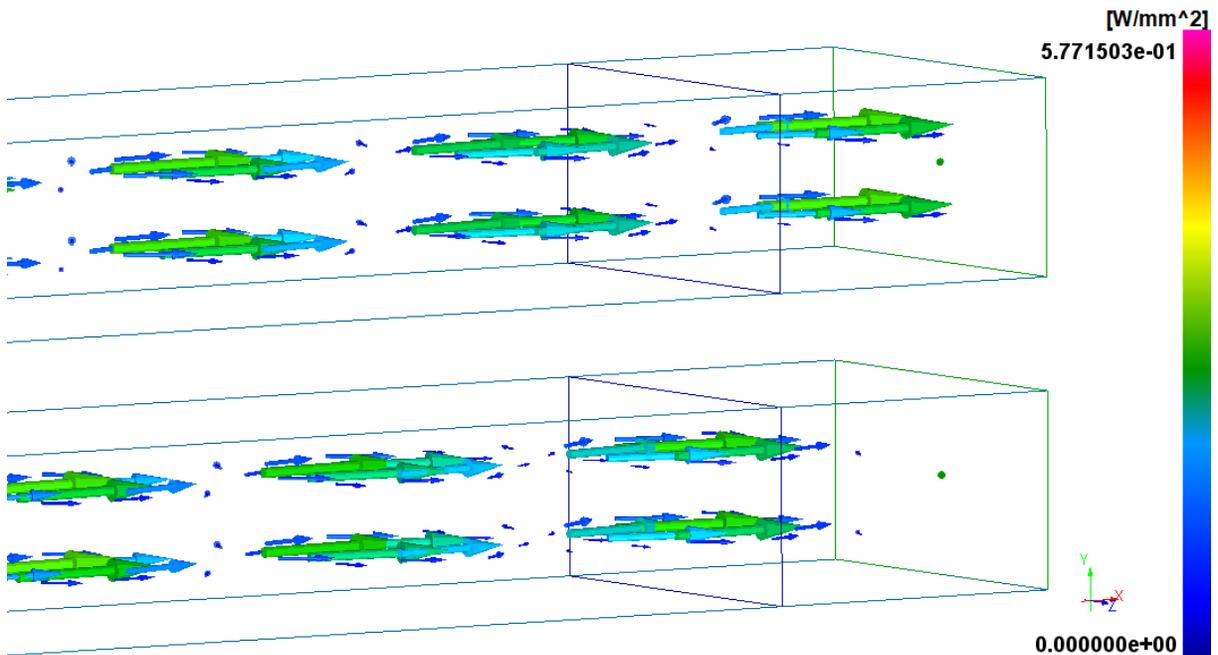
**Fig. 6** Distribution of momentary Poynting vector at 86.74 GHz: a) full structure. b) zoom on ports 2 and 4.
